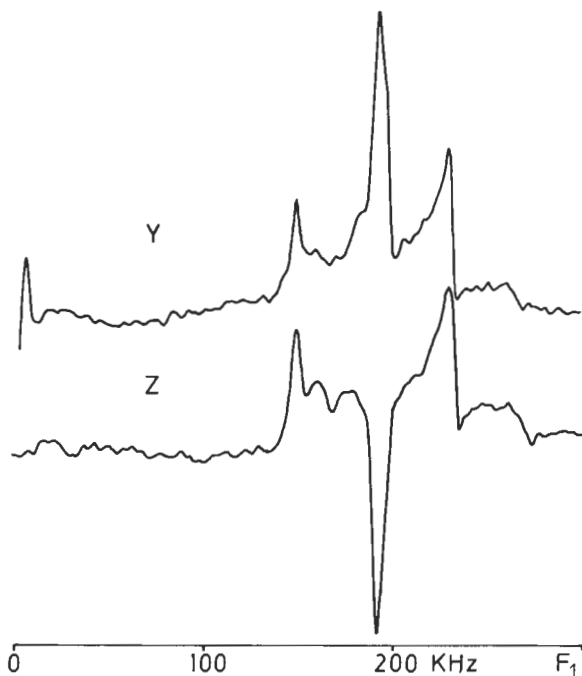
FIG. 8. The y and z components of the central transition magnetization of ^{23}\text{Na} ( I = \frac{3}{2} ) in \text{NaNO}_3 ( e^2qQ/h = 334 kHz (13)) at 53 MHz. The spin state evolution is determined by the x pulse ( \omega_{\text{RF}} = 180 kHz). The z component of the central transition magnetization is rotated into the x, y plane selectively with an additional attenuated 90^\circ pulse ( \omega_{\text{RF}} = 10 kHz) of the same frequency. The experimental spectra were registered on Bruker Physik CXP-series NMR spectrometers at 4.7 and 8.4 T.
